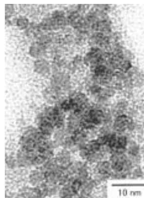
Fig. 6 TEM image of TiO 2 particles prepared by Ar 95%–O 2 5% gas mixture injection using a 532 nm wavelength laser
